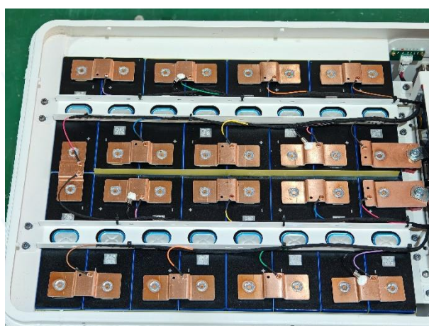
No.5.5-10 Inspection after test (No dust ingress)
