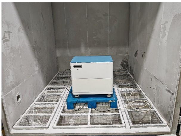
No.5.5-7 IP6X test (The degree of protection against the entry of solid foreign objects)
