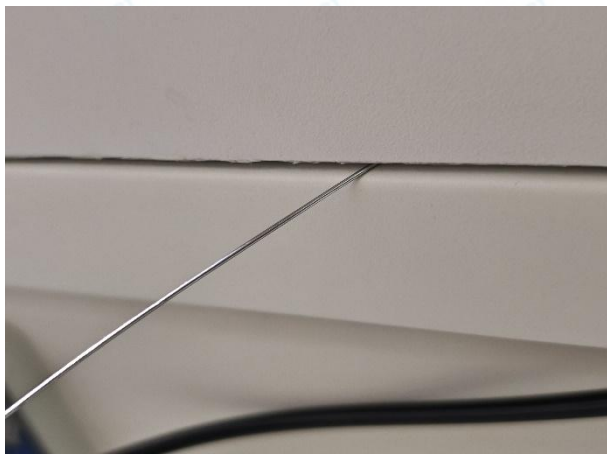
No.5.5-5 IP6X test (Degree of protection against access to hazardous parts)
