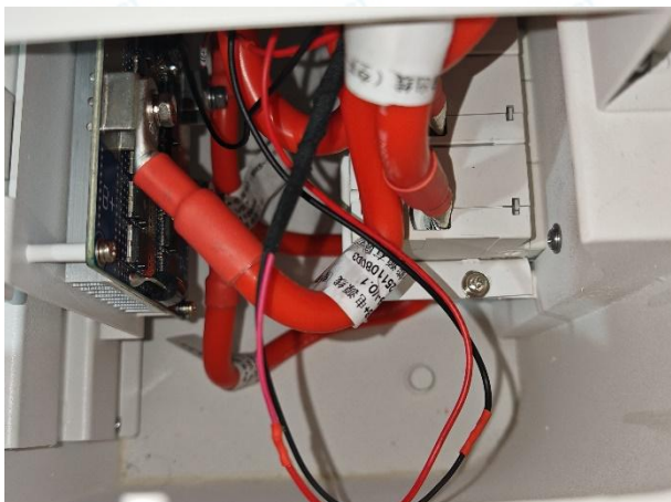
No.5.5-11 Inspection after test (No dust ingress)
