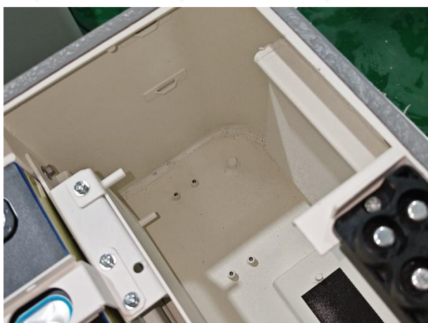
No.5.5-15 Inspection after test (No dust ingress)
