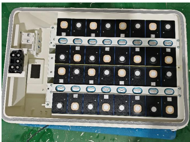
No.5.5-13 Inspection after test (Lower cavity)
