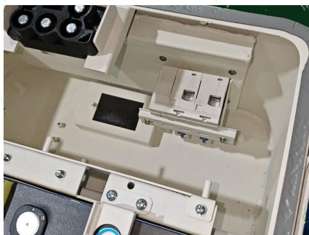
No.5.5-16 Inspection after test (No dust ingress)
