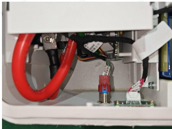
No.5.5-12 Inspection after test (No dust ingress)
