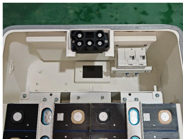
No.6.5-6 Inspection after test (No water ingress)
