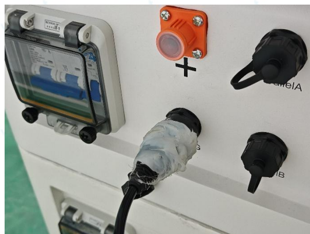
No.5.5-6 IP6X test (Place negative pressure on the specimen)
